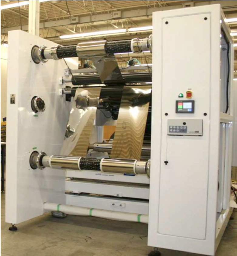
Web slitter Courtesy of Northfield Automation Systems
