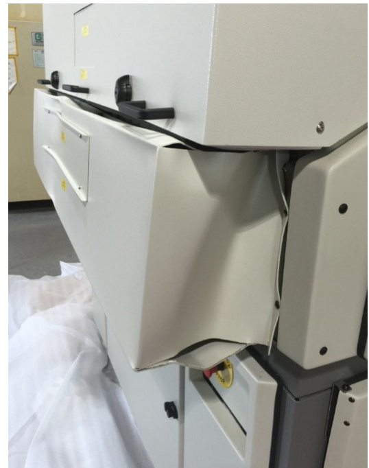
Poor handling during shipment can result in severe equipment damage
