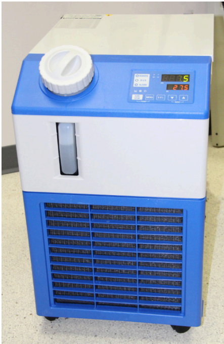
Example of laser chiller with water level gauge.
