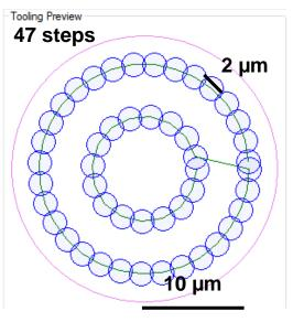
Effective Speed = 2 m/s Effective Acceleration (outer circle) =  $400,000 m/s^2$ Effective Acceleration (inner circle) =  $800,000 m/s^2$ Galvo Routing Max Speed ~ 0.4 - 0.5 m/s
